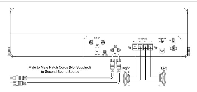
Aux Audio Input (LS9600UCDW/S Only): Left and right RCA type input jacks are provided on the back panel for connection to a second sound source such as a TV system or component cassette deck. Connect a stereo "male to male" patch cord to the units input jacks and then connect the remaining ends to the second sound sources output jacks.
